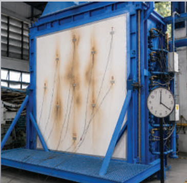
After for Fire Test ( p ) 4:00 hr
