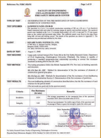
Fire Testing on Wall 50 mm.
